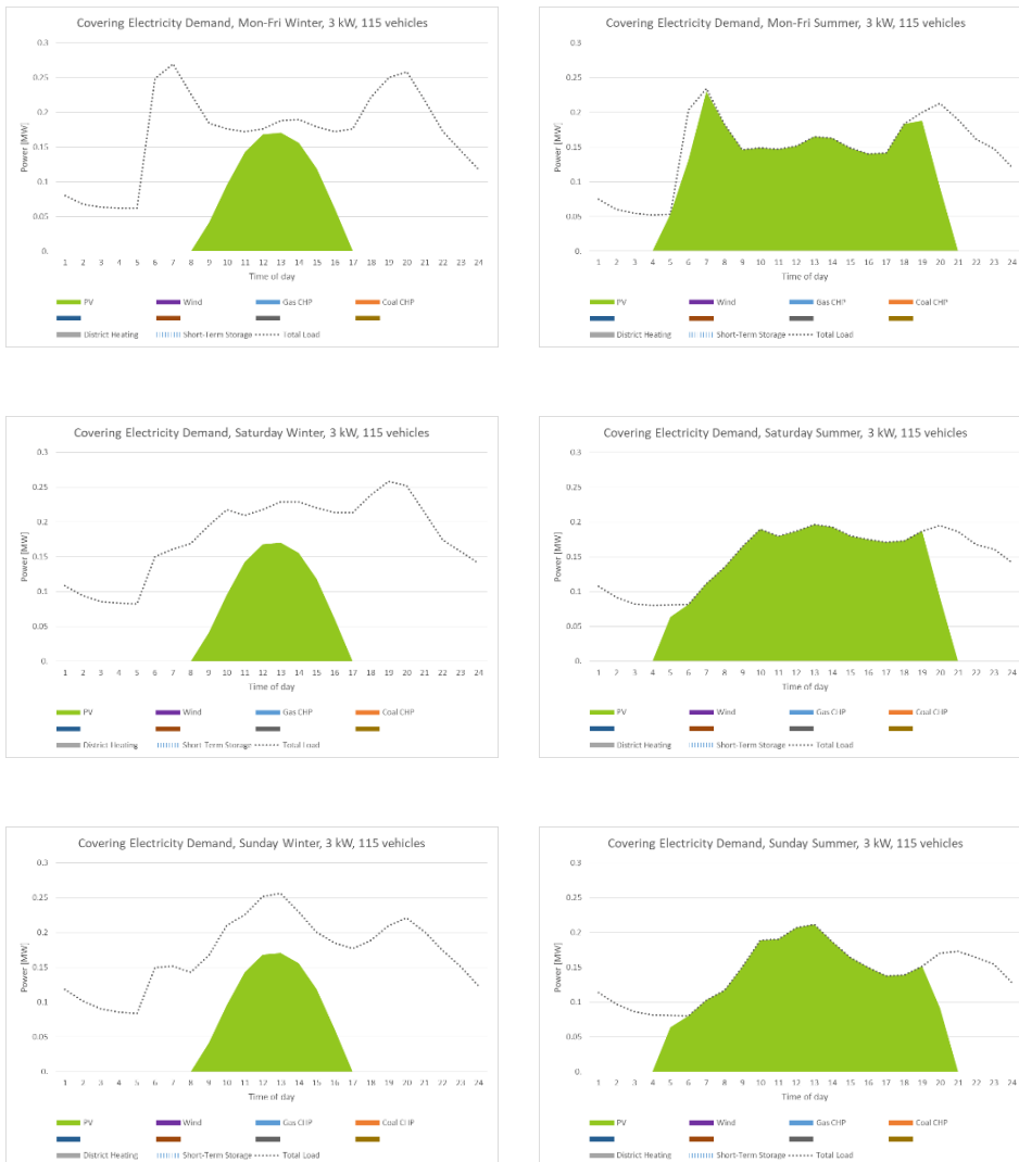
Fig 3.: Load curve for the block with EV charging, 3 kW chargers, 50% EV
