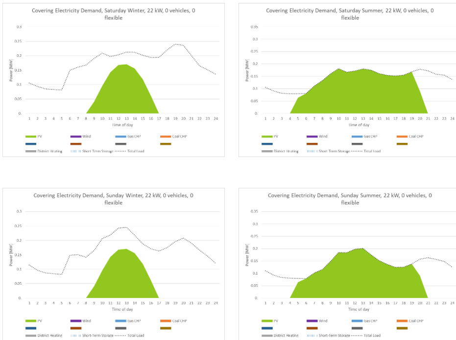
Fig 1.: Load curves for the case study block including all energy services except EV charging
